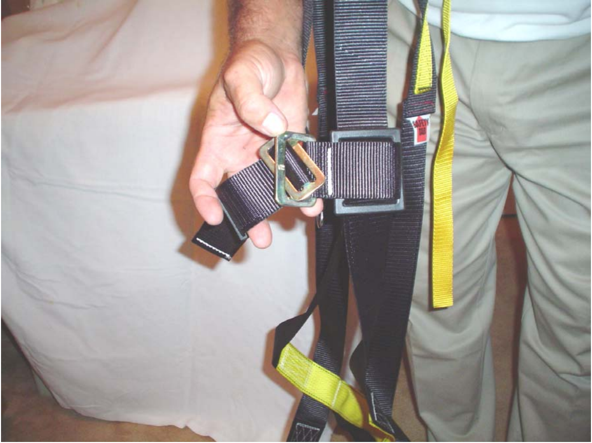
How buckle fits together leg and chest
